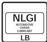
**Note B:** Not recommended for unheated shops where centralized automatic dispensing systems or long manual grease runs are the preferred method of lubrication and normal operating temperatures are consistently below -7°C (20°F).
